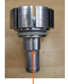
Rotor within tolerance  $\rightarrow$  Remain in machine
